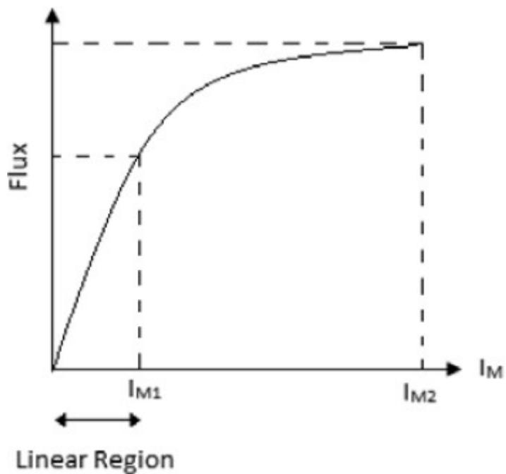
Figure 1 - Magnetization curve of current transformer
